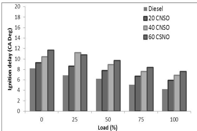
Fig. 5: Ignition delay vs. Load
