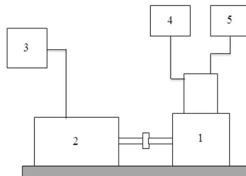
1. Engine, 2. Dynamometer, 3. Dynamometer control, 4. Air box, 5. Fuel tank
