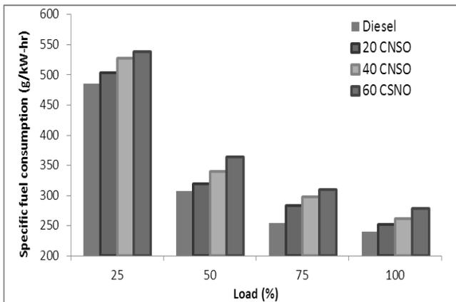
Fig. 3: Specific fuel consumption vs. Load
