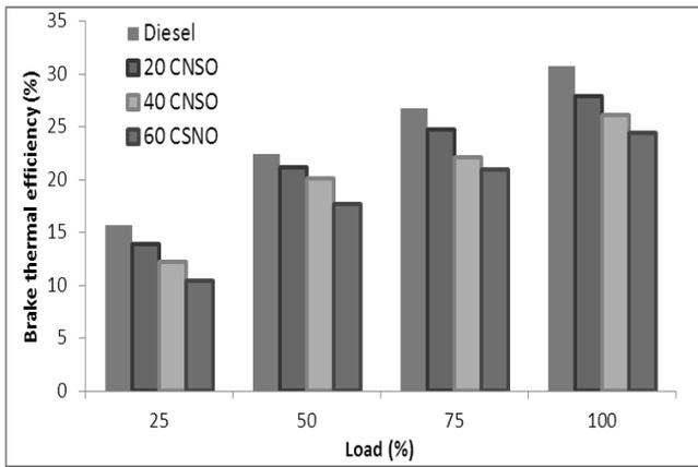
Fig. 2: Brake thermal efficiency vs. Load
