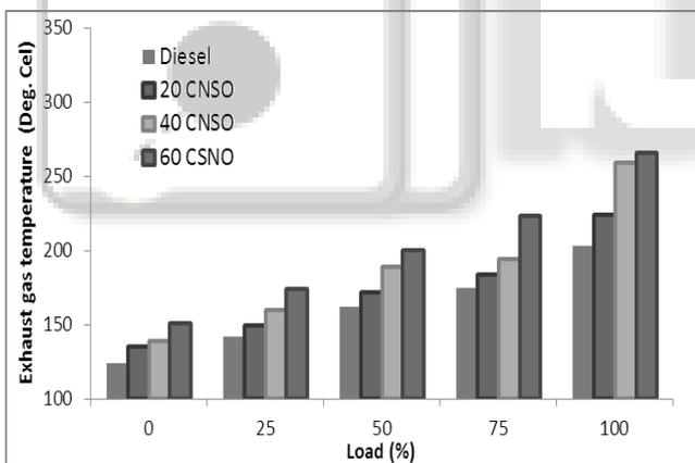
Fig. 4: Exhaust gas temperature vs. Load
