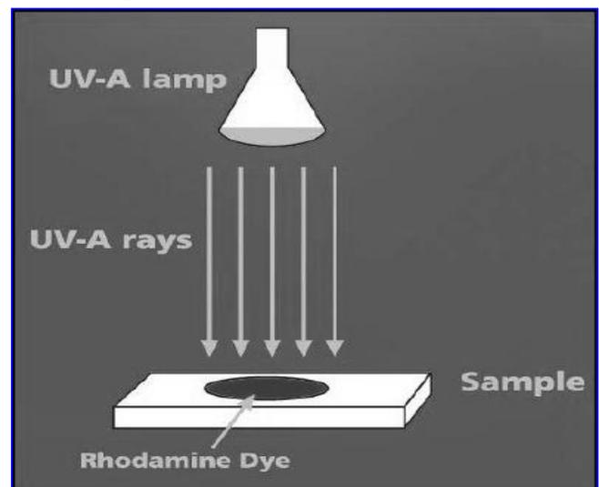
Fig. 3: Self – cleaning Measurement [10]
