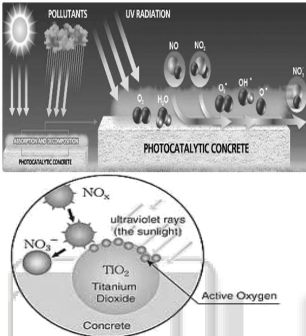
Fig. 2: Process between concrete pavement and UV rays and other oxide [4]
