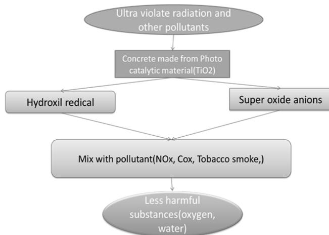
Fig. 3 Photocatalytic process
