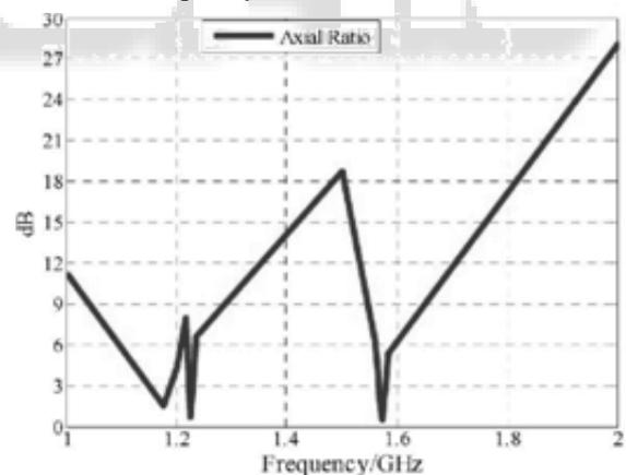
Fig. 5: Simulated axial ratio of the proposed antenna.<sup>[4]</sup>
