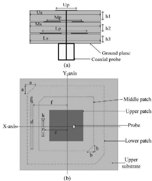
Fig. 6: Geometry of Triple Band-frequency patch antenna [5] The GPS performance in both L1 and L2 bands has a circular polarization (CP) with a broadside radiation, pattern while a linear polarization (LP) is achieved in GSM 1800 band.
