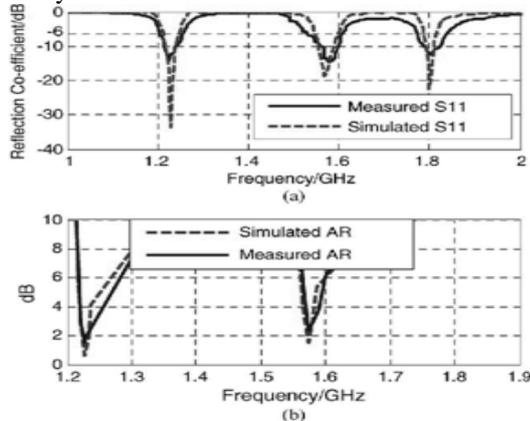
Fig. 7: Measured and simulated reflection coefficient and axial ratio of the pro-posed antenna: (a) measured and simulated reflection coefficient and (b) measured and simulated axial ratio. [5]
