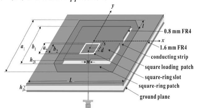
Fig. 2: Geometry of Dual band-frequency patch antenna<sup>[3]</sup>
