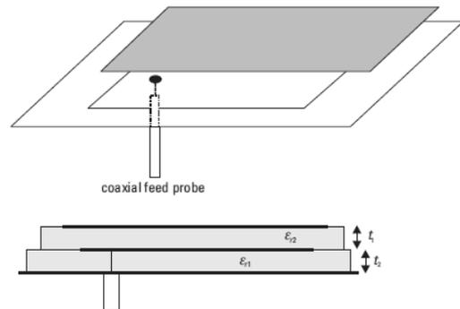
Fig. 1: Stacked Patch Configuration
