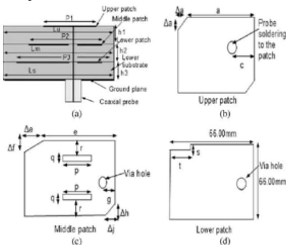
Fig. 3: Geometry of the proposed stacked patch CP antenna showing: (a) side view; (b) upper patch; (c) middle patch; and (d) lower patch.<sup>[4]</sup>
