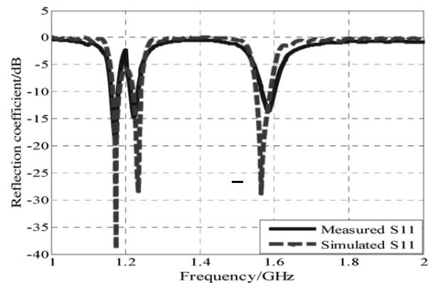
Fig. 4: Measured and simulated reflection coefficients of the proposed antenna.<sup>[4]</sup>
