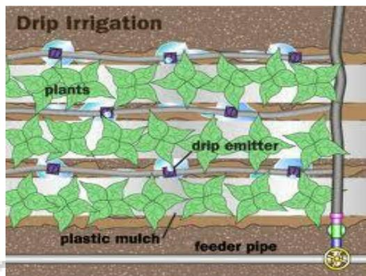
Fig.3. Drip Irrigation working arrangement
