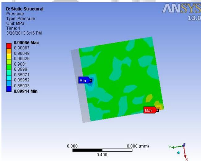
Fig. 5 contact pressure of bodies of  $5 \mu\text{m}$  roughness
