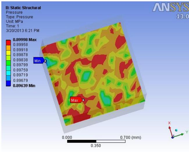
Fig. 4 contact pressure of bodies  $1 \mu\text{m}$  roughness
