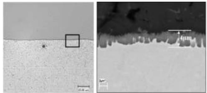
Fig. 6: SEM Showing an inter-metallic phase formation < 4μm in thickness
