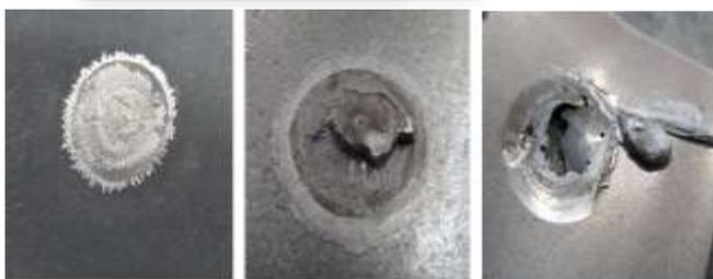
Fig. 3: Fracture behavior of a sample with 8 kA (left) and 11 kA (middle) and aluminium expulsion at 12.00 kA (right)
