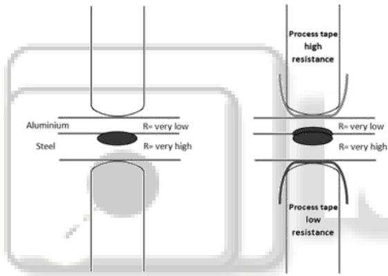
Fig. 1: RSW without process tape (left) and with process tape (right) for two different materials
