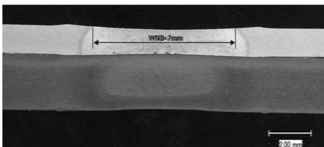
Fig. 5: 2 mm zinc coated DP600 steel to 1 mm aluminium alloy 5182
