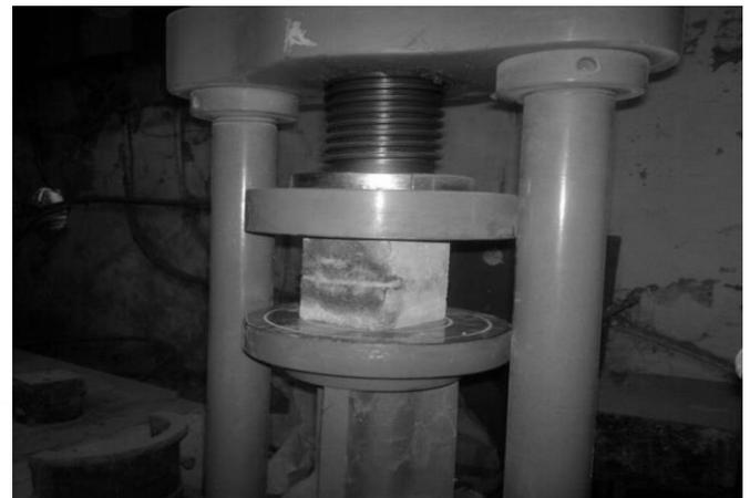
Fig.1. compression test
