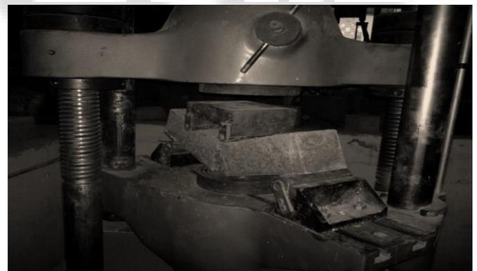
Fig 2. Flexural test
