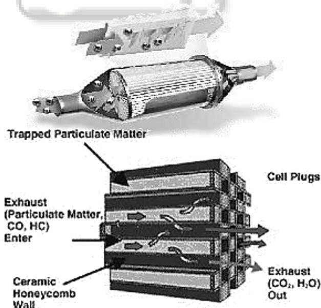
Fig. 1: construction details of DPF
