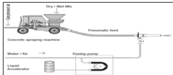
Fig. 2: Thin flow process for dry/ wet mix
