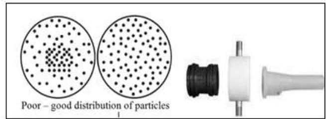
Fig. 4: Distribution of particles & Nozzle
