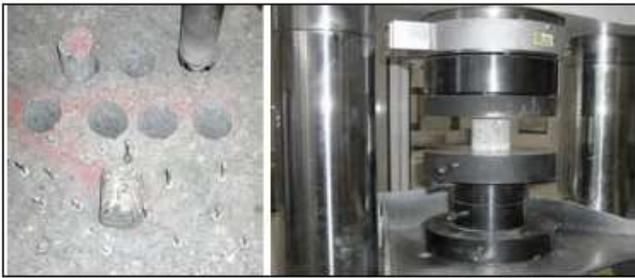
Fig. 9: Drilling of core sample & Compressive strength measurement
