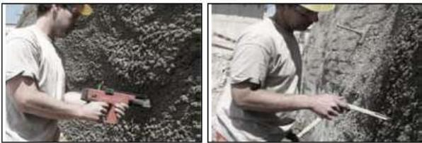
Fig. 8: Stud driving method: Penetration & measurement
