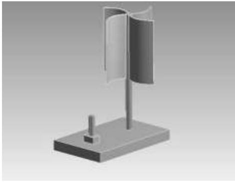
Fig. 2: Schematic Diagram of VAHT
