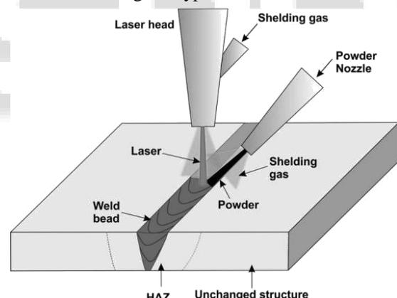
Fig. 2: Schematic of Laser Welding
