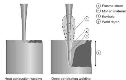
Fig. 1: Types of Welds
