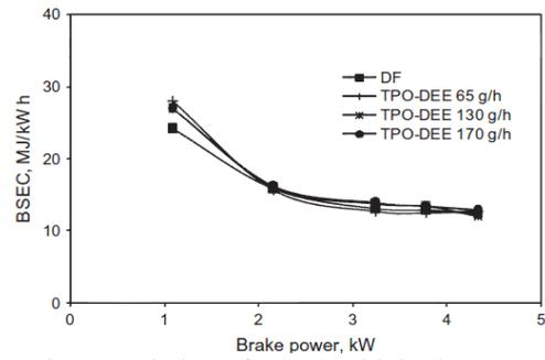
Fig.3. Variation of BSEC with brake power [3]
