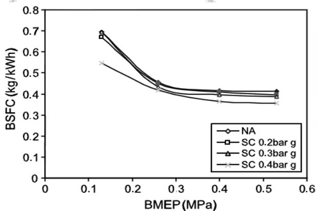
Fig.4. Performance comparison with and without supercharging [6]
