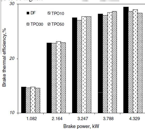
Fig.2. Variation of brake thermal efficiency with brake power [2]
