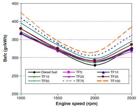
Fig.3. Variation of BSFC with engine speed for TF blends and diesel fuel [4]
