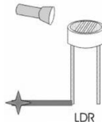
Fig. 4: Light Dependent Resistor Light Sensor [2]
