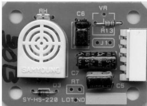
Fig. 5: SY-HS-220 Humidity Sensor [7]
