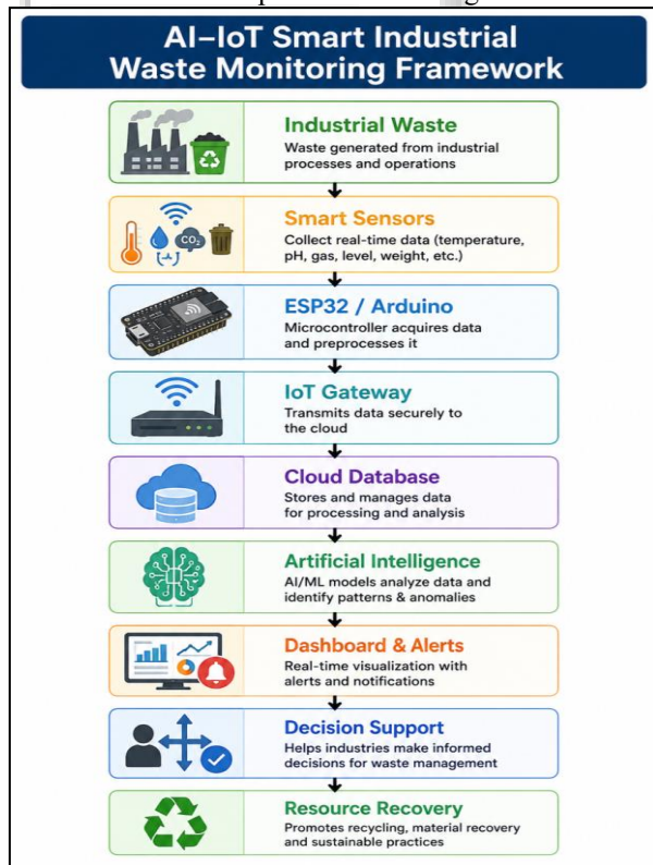
Fig. 2.1: AI-IoT Smart Industrial Waste Monitoring Framework
