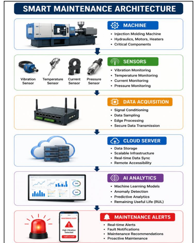
Fig. 3.1: Industry 4.0-based smart maintenance architecture developed for monitoring injection molding machine health.
