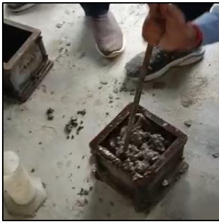
Fig. 7: Filling of concrete in mould
