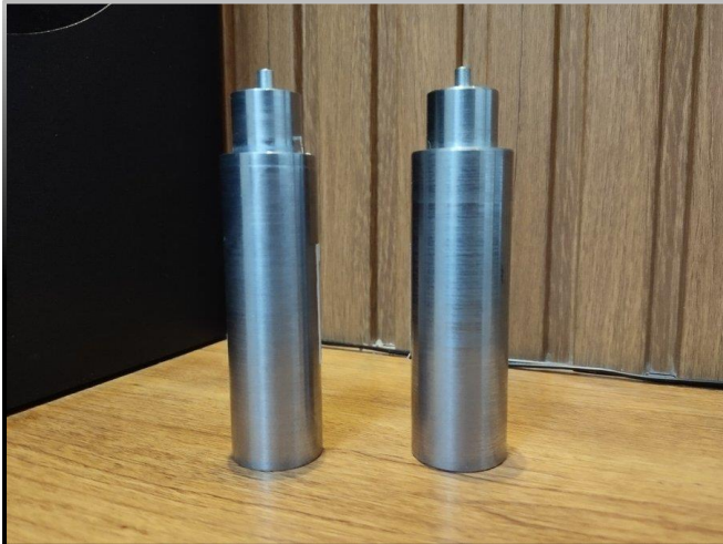
Fig. 2: Fabricated FSW Tools After Heat Treatment and Final Machining Cold Work Die Steel Tool (Left) and H13 Hot Work Tool Steel (Right)
