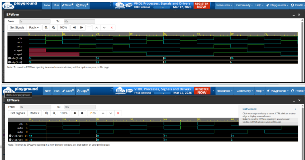
Fig. 2: Verilog simulation waveform showing clock, input signals, intermediate stages, and comparator outputs.
