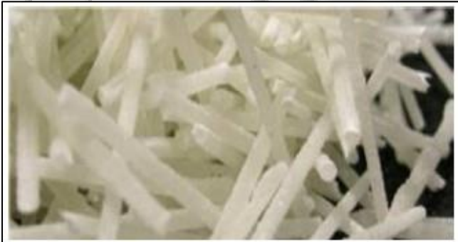
Synthetic Fibre used In Fibre Reinforced Concrete
