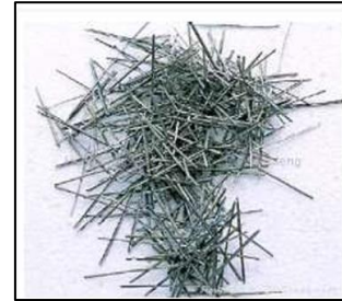
Steel Fibres Extracted from Binding Wire
