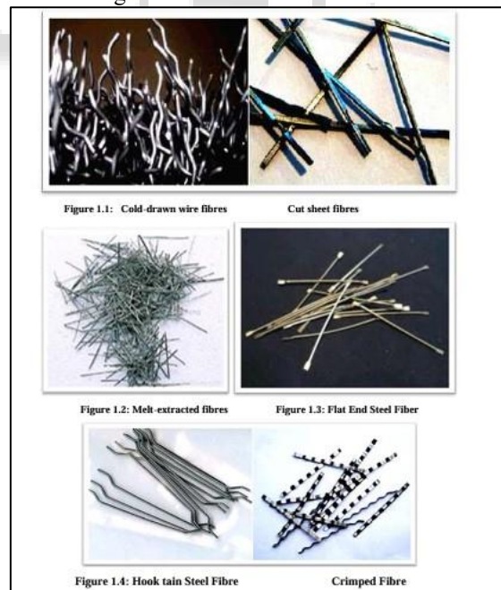
Different Types of Steel Fibre used in Steel Fibre Reinforced Concrete
