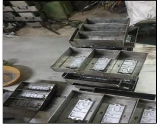
Fig. 3.6: Clay Brick Mould.
