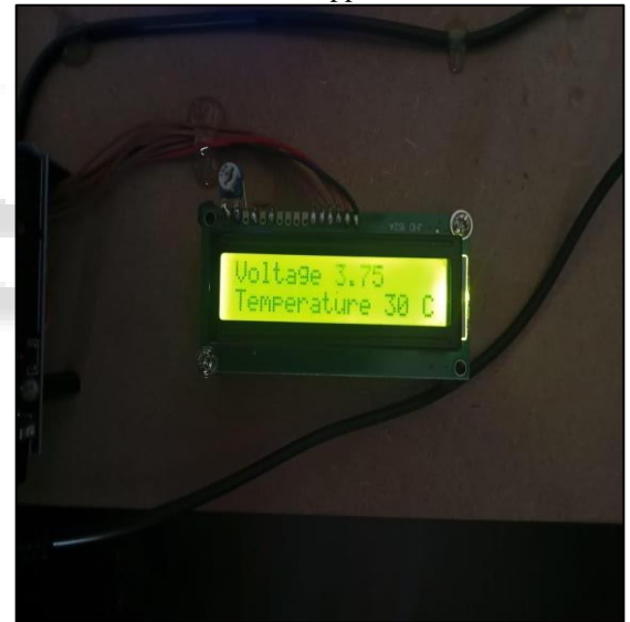
Fig. 5: Measurement of the Voltage and Temperature After Brake Applied.
