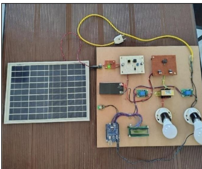
Fig. 4.1: Model of peer-to-peer energy exchange prosumer driven solutions for smart grid
