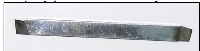
Fig. 3: Centrifugal cast tool after heat treatment [5]
