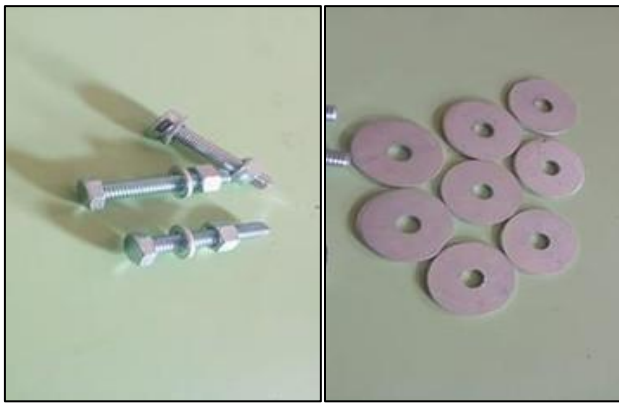
Fig. 3.6: Bolts and zinc plated MS plate round washer
