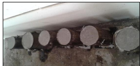
Fig. 8: Cylinder specimen casting
