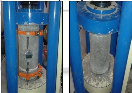
Fig. 10: specimens are tested for Young's modulus
