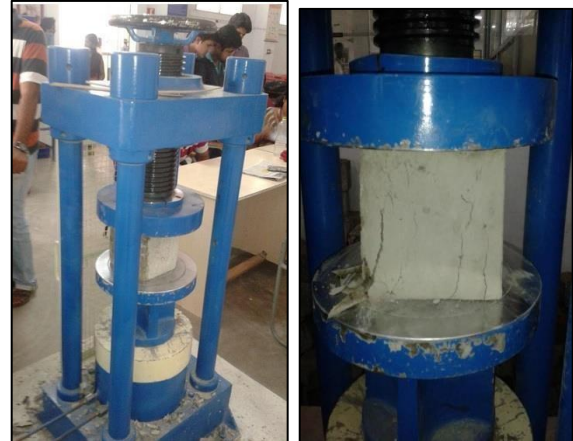
Fig. 6: Samples testing with a compression testing machine
