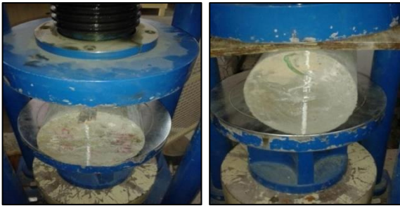
Fig. 9: Testing of cylinder specimens in a compression testing apparatus
