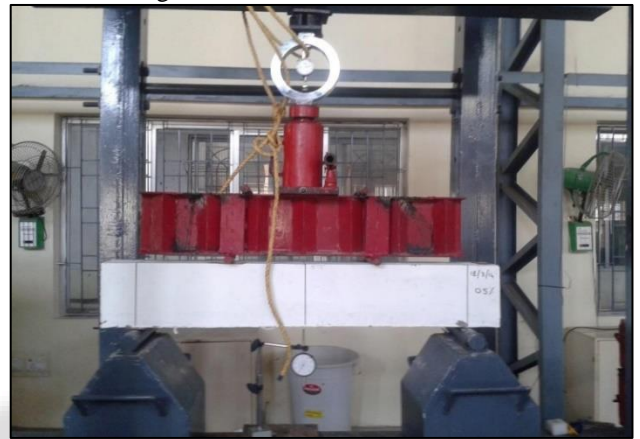
Fig. 13: PET 0.5% Reinforced Beam Testing
