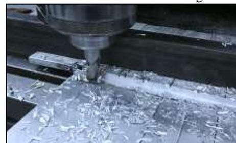
Fig. 1: Weld removal by vertical milling machine
