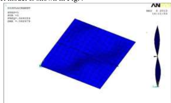
Fig. 4: Buckling mode shape for P1R model
