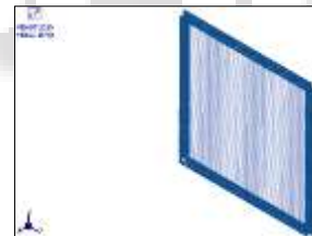
Fig. 1: Modeled composite laminated plate with all edges simply supported
