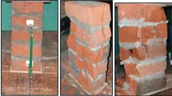
(a) Prism sample (b) During Compression (c) Loading after cracking
