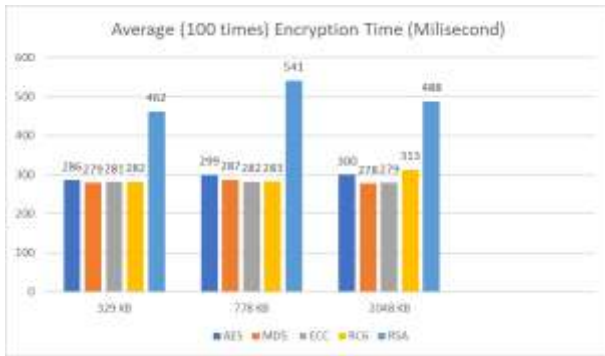
Fig. 2: Encryption time of different algorithm (column based)
