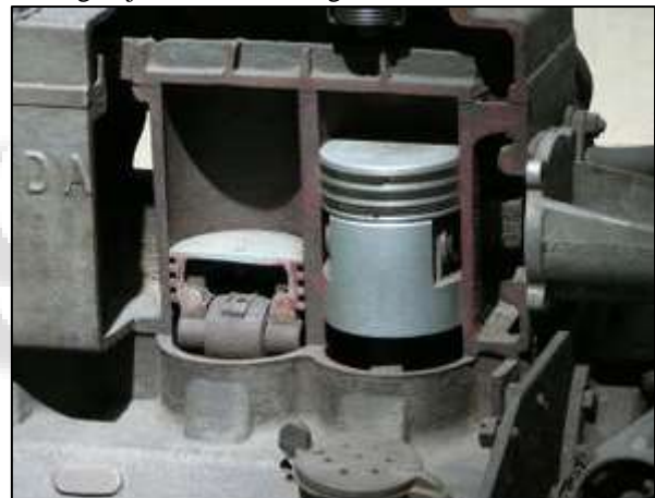
Fig. 1.1: A piston contained inside of a cylinder, used within a sectioned gasoline engine
