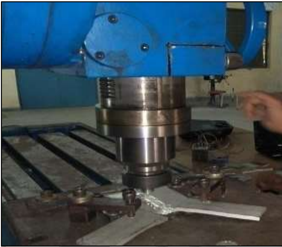
Fig. 1: Vertical milling machine for friction stir processing.
