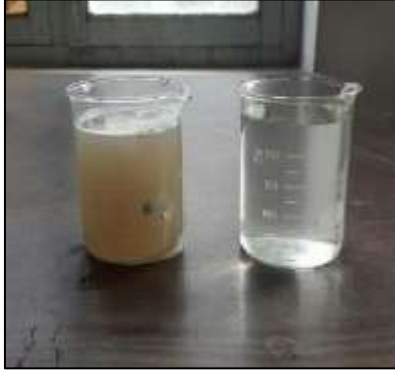
Fig. 4: Wastewater before treatment and the treated water
