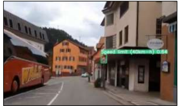
Fig. 5: Speed Limit 40 km/h Sign Detected.
