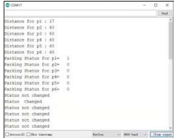
Fig. 6: Raspberry Pi integrated Arduino monitor display
