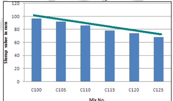
Fig. 12: Slump value in mm for C1 (ordinary Portland cement) category mix
