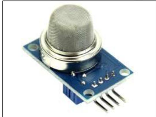
Fig. 5: MQ-6 sensor
