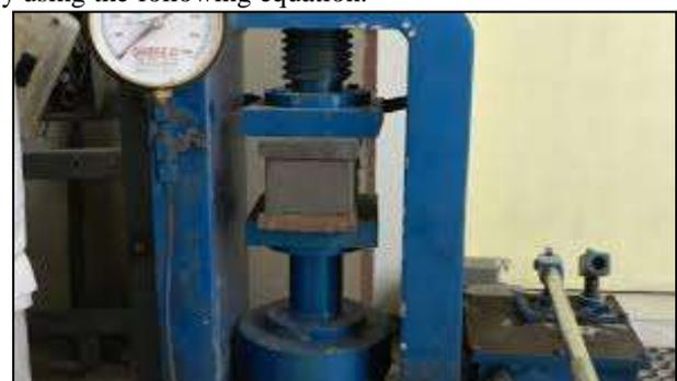
Fig. 1: Compressive Strength Testing
