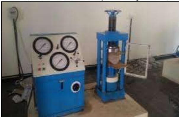
Fig. 2: Split tensile strength testing
