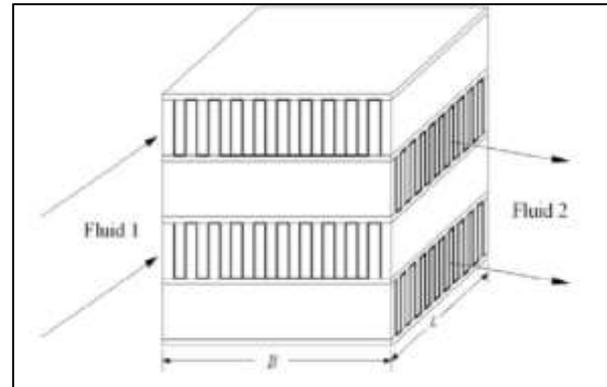
Fig. 1.5: Plate Fin Heat Exchanger
