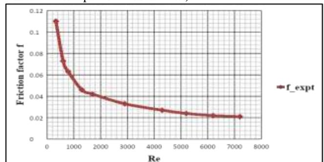
Fig. 5.2: Plot of Reynolds Number Vs Fanning friction factor f, determined experimentally
