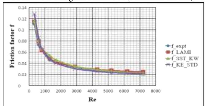
Comparison of experimental and numerical values for friction factor  $f$
