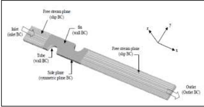
Fig. 3.3: Boundary conditions (BC) and extended flow volumes are included in the computational domain
