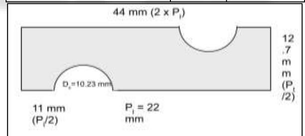
Fig. 3.2: The primary computational domain and geometric parameters of the heat exchanger
