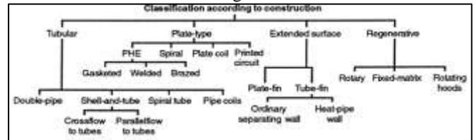
Fig. 3.1: Classification of Heat Exchangers
