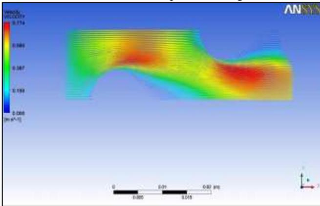
Velocity vector for inlet velocity 0.3 m/s, SST k-omega flow model
