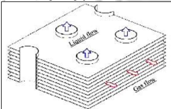
Fig. 1.10: Typical fin-and-tube heat exchanger section with staggered tube arrangement
