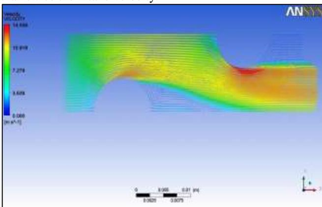
Fig. 5.4: Velocity vector for inlet velocity 6.2 m/s, SST k-omega flow model
