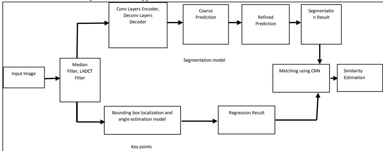
Fig. 1: Architecture of the aircraft recognition framework
