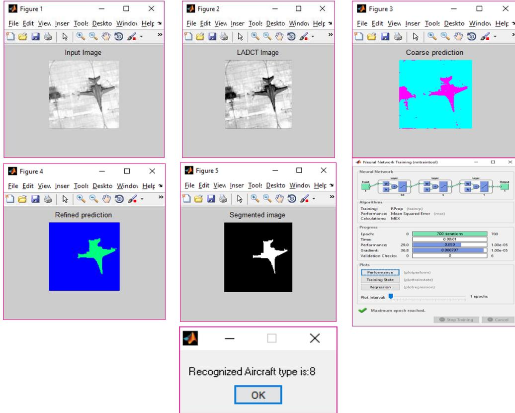
Fig. 3: The recognition result using LADCT filter.
