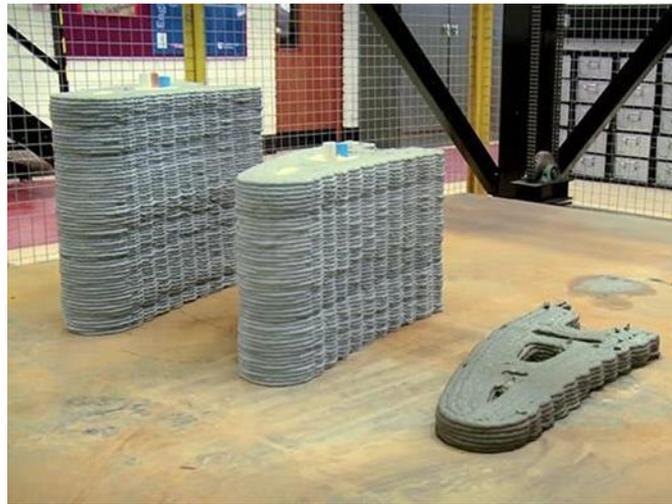
Fig. 3: Section Printed by Freeform Construction
