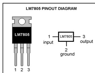
Fig. 5: LM7805 Pin diagram
