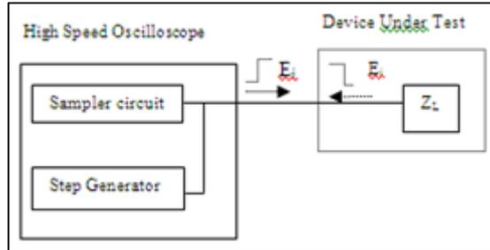
Fig. 2: Functional block diagram of TDR
