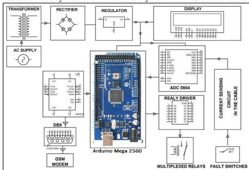
Fig. 3: Block diagram of underground cable fault distance conveyed over GSM
