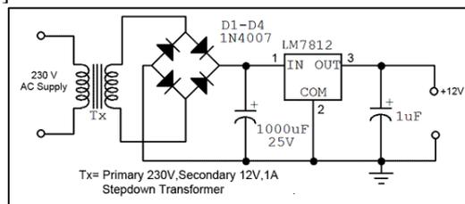
Fig. 4: Power supply of circuit
