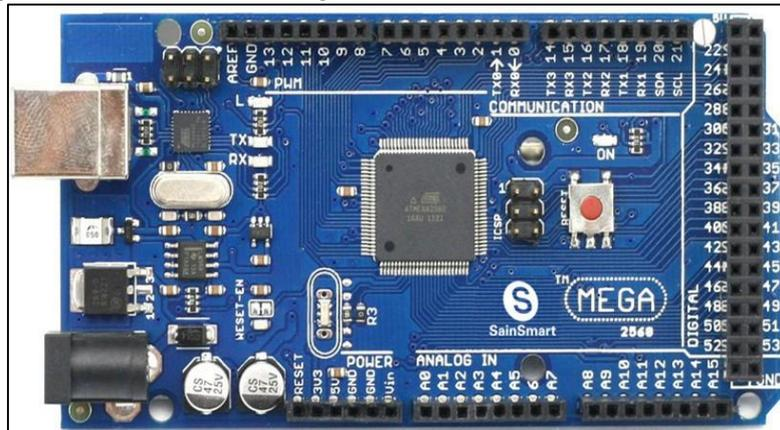
Fig. 6: Arduino Mega 2560
