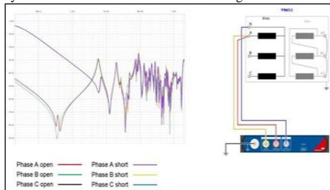
Fig. 5: Typical response of an end to end short circuit test (left) and connection diagram (right)
