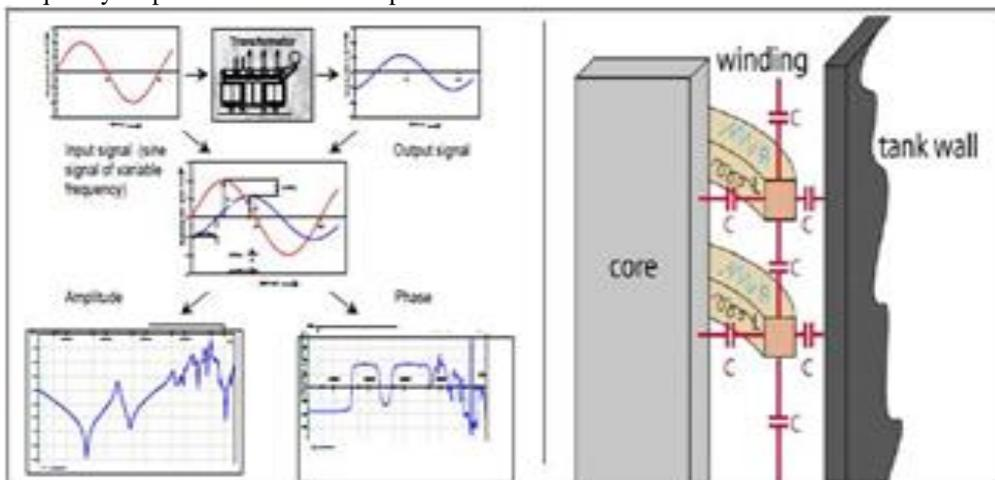
Fig. 1: Principle functioning of SFRA (in left) and simple network behavior of transformer active part (in right)
