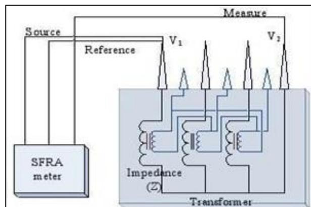
Fig. 3: A typical SFRA test connection
