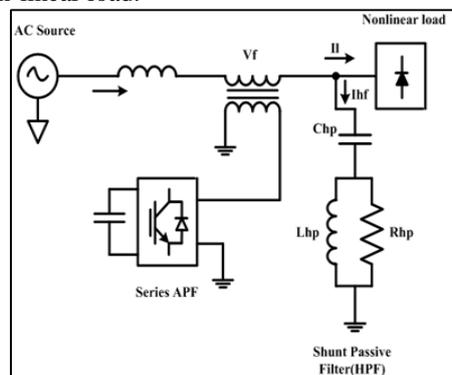
Fig. 7: Hybrid Active Filter configuration 1
