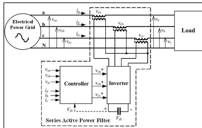
Fig. 3: Series Active Power Filter
