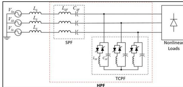
Fig. 6: Hybrid Passive Filter
