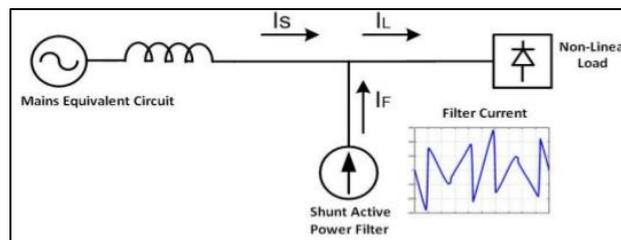
Fig 1: Shunt Active Power Filter
