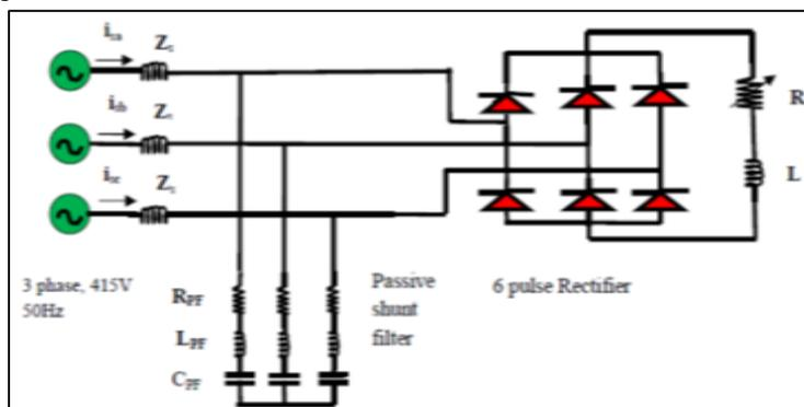
Fig. 5: Shunt Passive Filter
