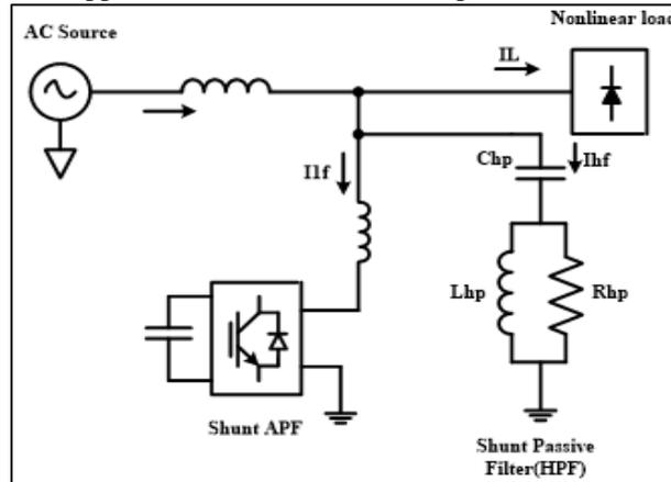
Fig. 8: Hybrid Active Filter configuration 2.
