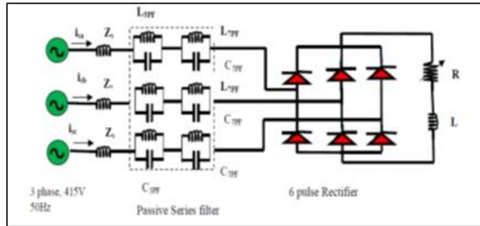
Fig. 4: Passive Series Filter
