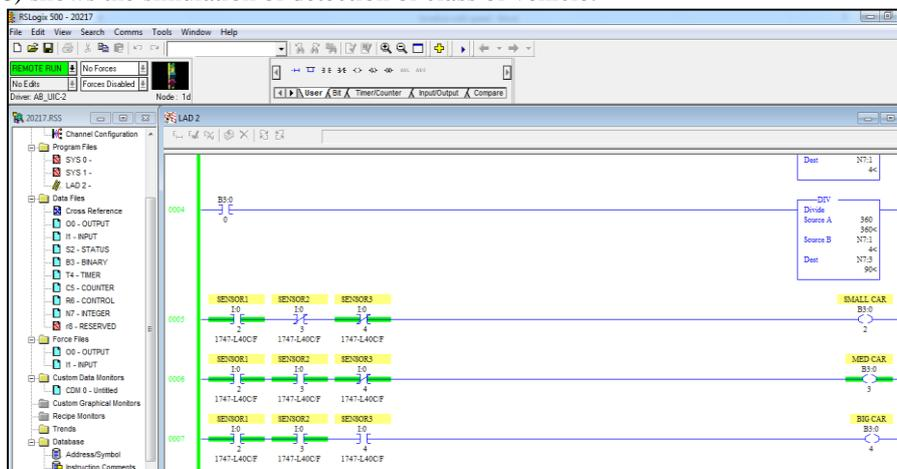
Fig. 8: Class of Vehicle Detection in Rslogix500
