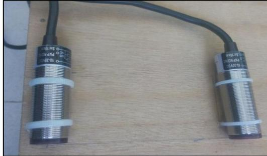
Fig. 2: Photoelectric Sensors
