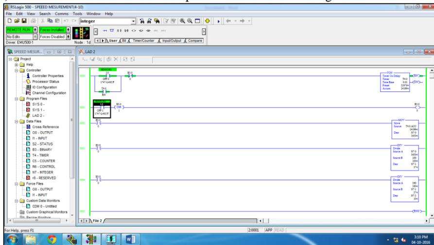
Fig. 7: Vehicle Speed Measurement In Rslogix500
