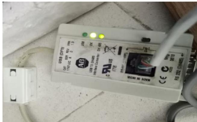
Fig. 3: Dh-485 Link Coupler of 1747-L40c(Ab Slc-500)
