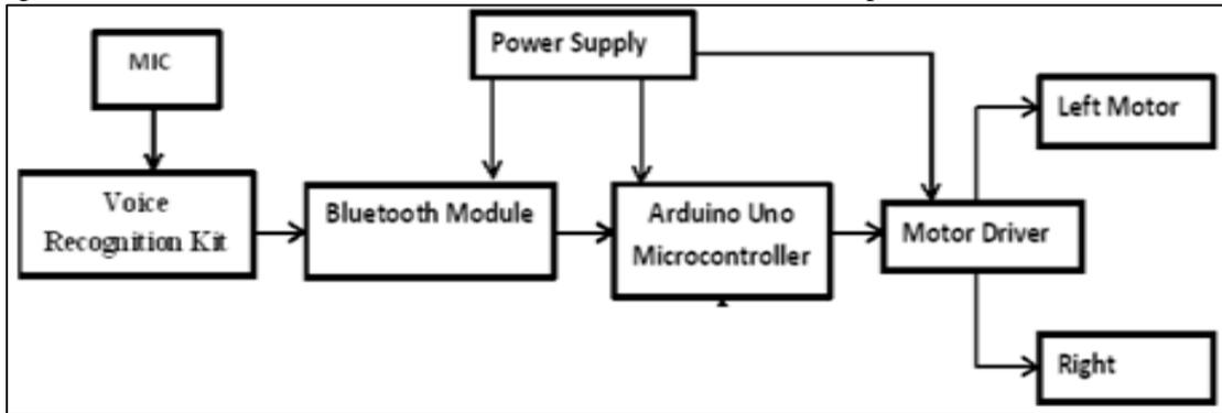
Fig. 1: Block Diagram
