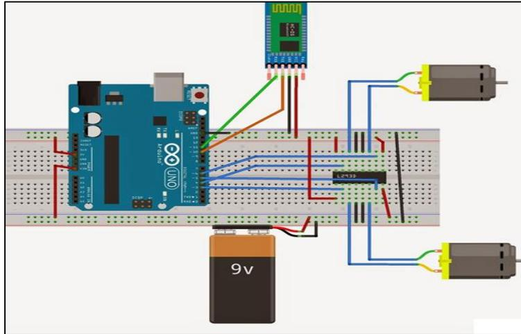
Fig. 3: Main Circuit Diagram
