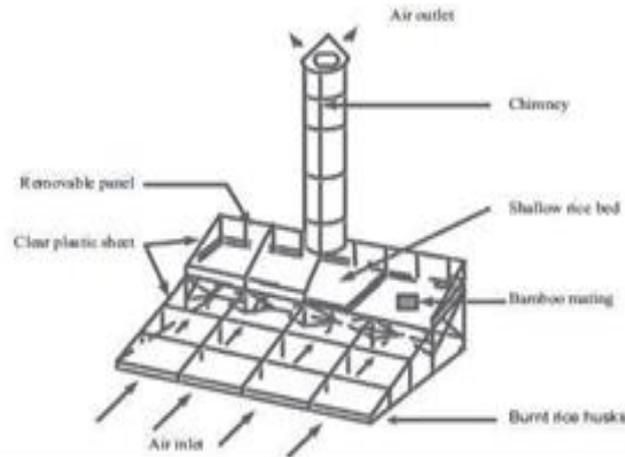
Fig. 3: Mixed mode solar dryer
