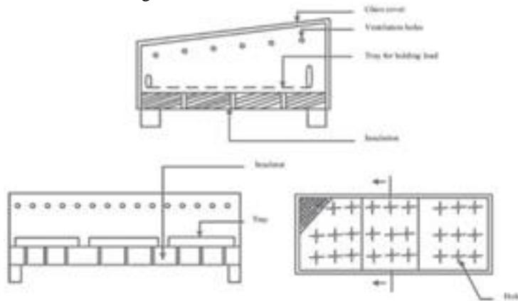
Fig. 1: Direct Solar Dryer
