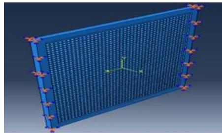
Fig. 12: Boundary conditions keeping both the sides fixed
