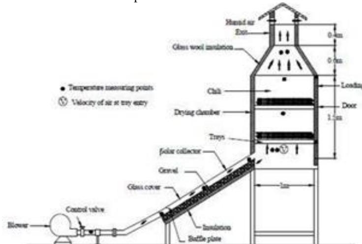
Fig. 2: Indirect Solar Dryer
